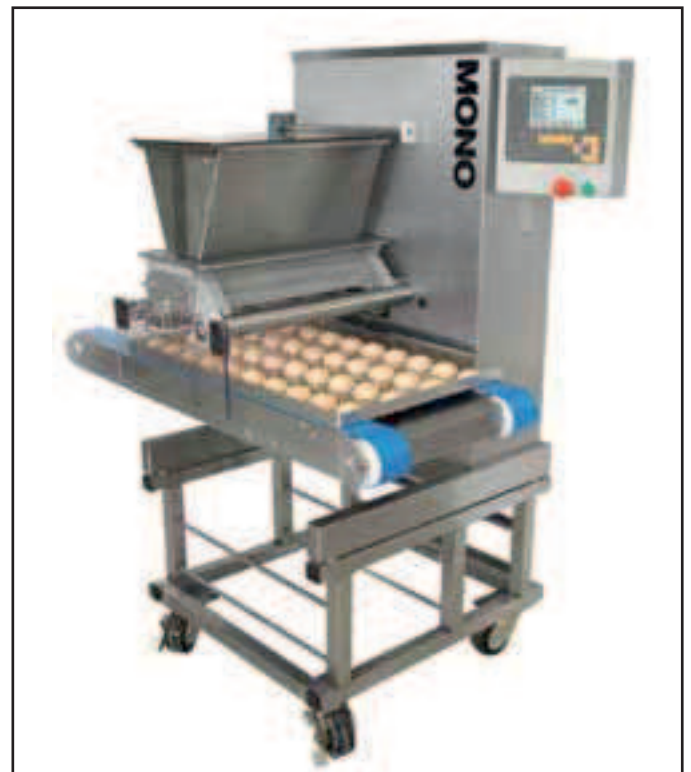
Photo of the dough depositor machine with the TRM 3 axis motion controller & HMI.
